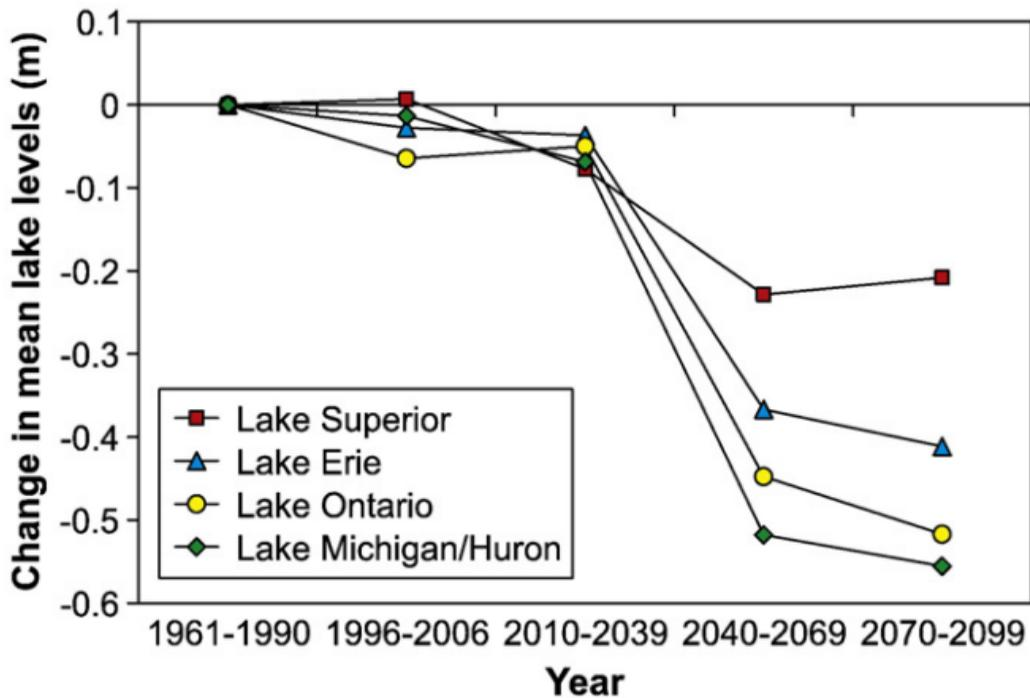
**Fig. 10.** Average Great Lakes levels depend on the balance between precipitation and corresponding runoff in the Great Lakes Basin and evaporation and outflow. **The SRES B1 lower emissions scenario with less warming (not shown) projects little change in lake levels over the coming century.** Under the SRES A1fi higher emissions scenario (shown here), decreases on the order of 0.5 up to nearly 2.0 ft are projected towards the end of the century.
